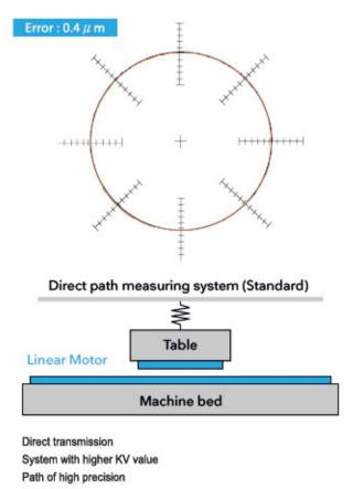
No backlash Source by: Siemens laboratory testing
